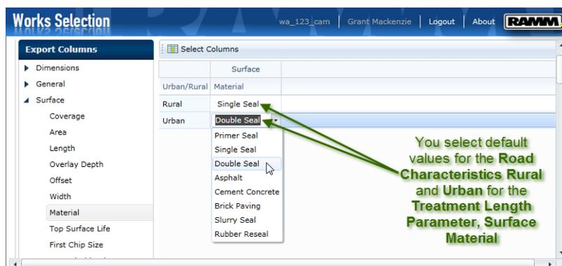
An example could be if you have both Rural and Urban Roads in your Network which mostly have different Surface Materials. So you would define two different Surface Material defaults being, for instance Single Seal for Rural and Double Seal for Urban.
