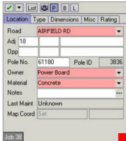
This screen shows the details of an asset - for example its different components, its location, whether it was replaced or updated recently.
