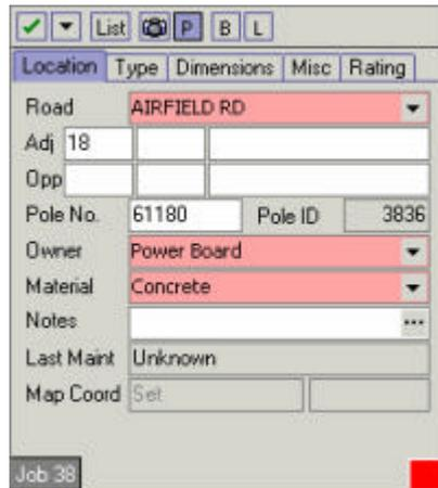
An asset may have different components: note the **P**, **B** and **L** icons. These represent Pole, Bracket and Light, and change according to the asset details currently being shown (if you're viewing Signs data, for instance, an **S** will appear instead).
